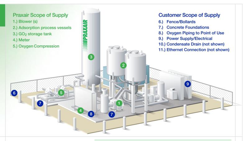
For customers needing up to 135 tons per day of oxygen, the ideal supply is Praxair's VM80 XL. The VM80 XL is a vacuum pressure swing adsorption (VPSA) plant that consists of a feed blower, sieve beds, vacuum blowers, surge tank and silencers. The system is designed and shipped on five skids – allowing very rapid field installation and minimum disruption to your site. Product delivery pressure is tailored to each customer's unique requirement.
