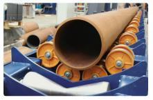
**ROLLER BED** A roller bed is used for pipe support. Tandem wheels prevent vibration during cutting.
