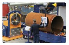
**THREE-JAW CHUCK** Comes standard to ensure precision pipe rotation during the cutting process.
