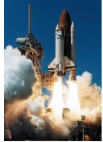
Helium is used to purge and pressurize liquid hydrogen fuel systems in rockets and spacecraft (photo courtesy of NASA).
