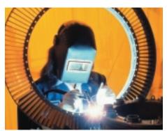
Gaseous helium is an ideal shielding gas for welding stainless steel, aluminum and other metals.
