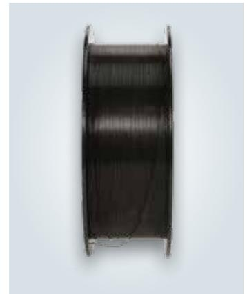
ADVANTAGE™ E70C-6M metal-cored wire is formulated for use with argon/CO<sub>2</sub> blends and designed for flat and horizontal position welding of carbon steel. It is level wound and features excellent feedability, good penetration and wetting, a smooth arc and high deposition rates.
