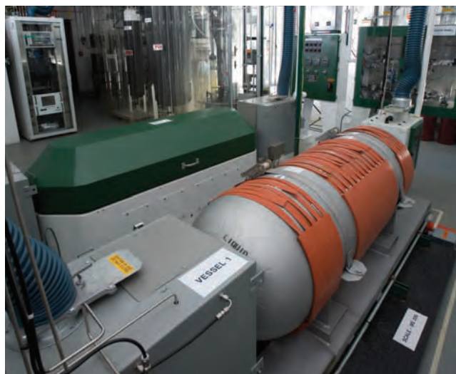
▲ Enclosed heating system (left) and silicone rubber heat system (right)
