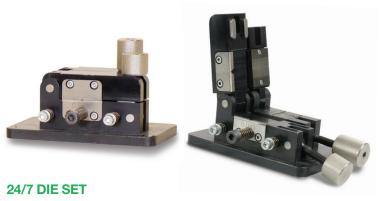
With shaving plates available for many wire diameters, the 24/7 die set ensures a consistent diameter across the welded seams when drums are joined together by removing the resultant flash and any burrs from the welding process.
