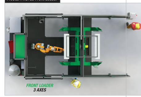
ProStar's PRSFL3 uses 360° single-axis positioners to support custom tooling bridles.
