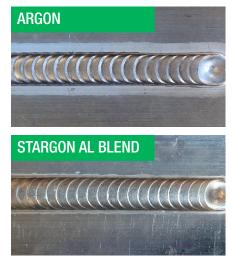
Welds made with *Stargon* AL gas blend result in a smaller cleaning zone with a smoother weld surface.
