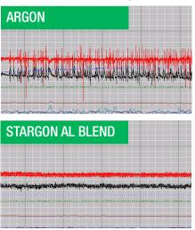
*Stargon* AL gas blend provides improved stability when compared to argon, as seen in the arc monitoring signals above.
